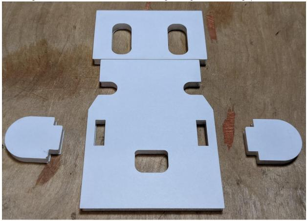
Glue the tabs into the fuselage hatch, using hot glue underneath the tab bonding areas, and on the interior of the tabs as shown.
