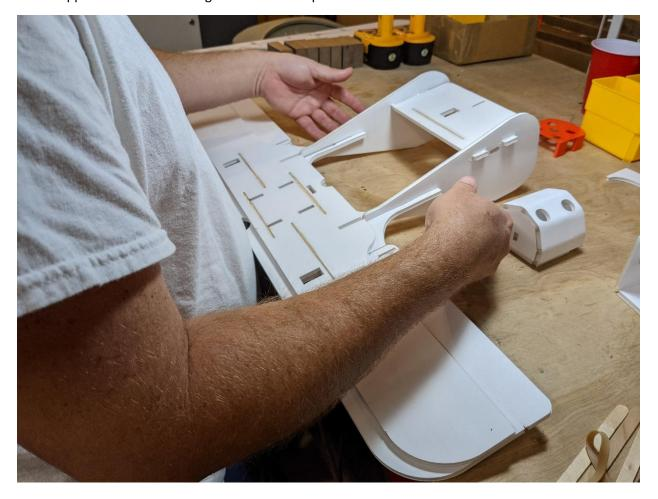
At this point I apply glue inside the upper wing surface alignment channels and then slide the vertical stabilizers the rest of the way into position.
