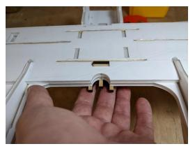
Insert the Alignment Pin and Motor Mount into the Wing assembly as shown. They are glued in on the lower wing skin. The Alignment Pin is protruding through the upper wing skin.
