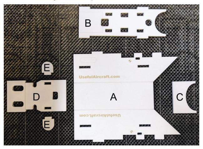
The fuselage subassembly consists of: (Parts labeled in photo above A, B, C, D, E)
