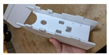
I place makers blocks on either side, and one in my avionics tray to allow the hot glue to cool while ensuring the fuselage is held square.
