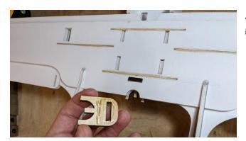
Apply glue to the remaining motor mount and glue it to the top of the upper wing skin.
