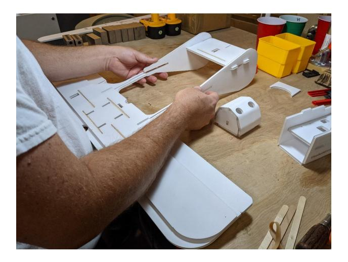
Ensure the hinge lines are facing down on both the tail and the wing. You should not be able to see the camber rib on the elevator. Don't apply hot glue until you're sure things are correct.
