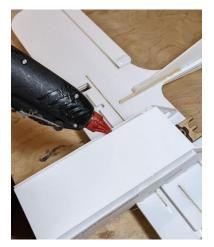
Run a bead of hot glue along the outer bottom edges of your fuselage. That connection between the lower skin and sidewalls of your airframe is only strengthened by this.
