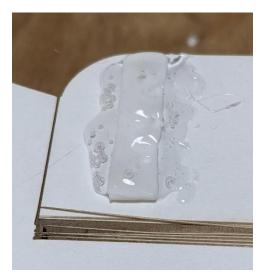
Flip the plane over and secure the control horns on the top side with additional hot glue.
