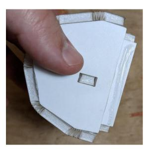
When installing the nose onto the airframe the first time, you may need to pinch the leading edge of the slip ring as it interfaces with the fuselage, as it's a snug fit. If things loosen up, you can apply a thin layer of hot glue to the exterior surface of the slip ring to make that fit snug again.
