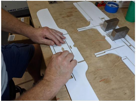
Apply weights to ensure the wing is flush to your build surface, and allow the Hot Glue to cool.
