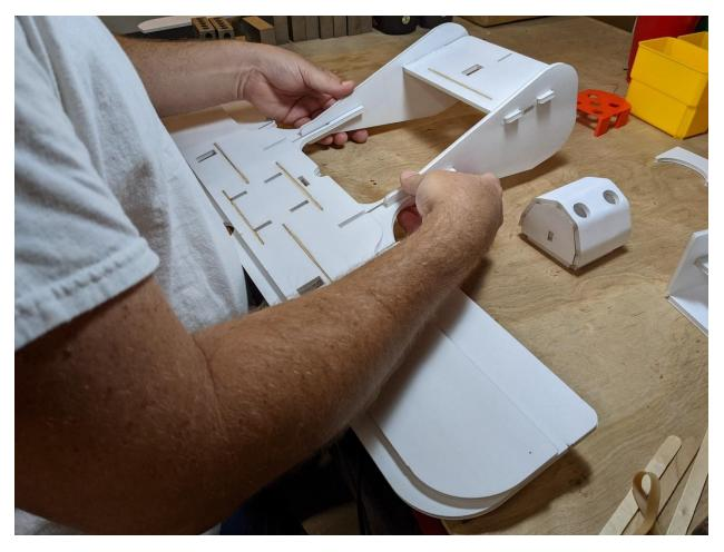
Align the parts and begin sliding them towards one another taking care to see where any binding is occurring and re-aligning the parts as they slide into one another.
