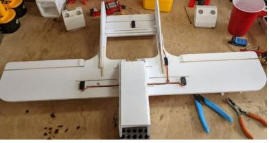
A small dot of hot glue is perfect for keeping servo wires in their conduits. When removing electronics from an airframe being recycled, isopropyl alcohol in high concentration makes hot glue fall right off.
