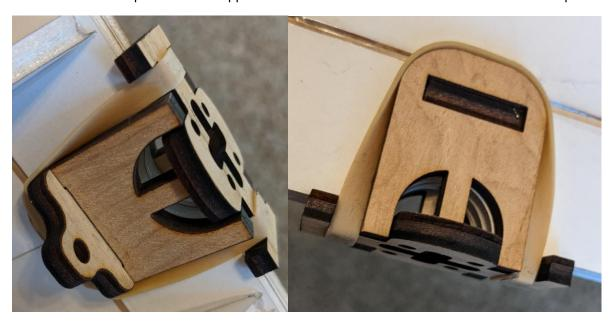
As this aircraft is a pusher design, the motor is pushed into the fuselage during forward flight. The rubber band allows the motor mount to have limited flex in the event of a prop strike and allows for easy motor changes. **There is no glue on the Motor Backplate.**
