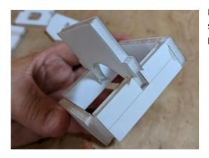
Next insert the camera platform. It is designed to be a snug fit. You may need to pinch the edges of the camera platform's interfacing tabs — and that's ok.
