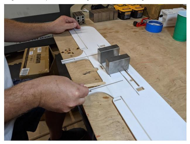
For the Upper Wing Skin, the procedure is the same. Apply hot glue into the fold seam.
