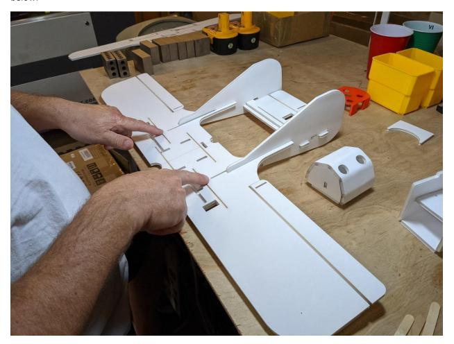
Apply glue to the flat side of a popsicle stick as shown in the photo below and install into the main wing assembly and to the interior surface of the vertical stabilizer. Ensure the popsicle sticks are well bonded to the vertical stabilizer and secure. The popsicle sticks are installed on the lower side of the wings, and the interior of the vertical stabilizers helping to strengthen the interface.
