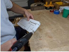
Run a bead of hot glue along the interior folds of the Upper Wing Skin as shown in the photos above.
