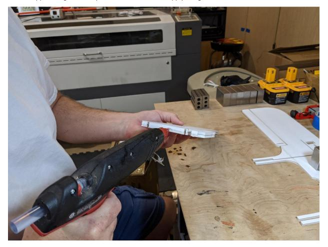
Lay the Upper Wing Skin Flat, and smear the Hot Glue along the fold line using a popsicle stick.
