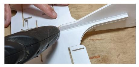
Apply glue beads in this manner to all interior and exterior joints surrounding each vertical stabilizer.
