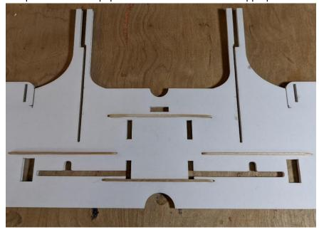
Before gluing – test fit the upper wing skin so you understand the alignment. Ensure the tab holes, servo mounting holes and wing tips are aligned. Correct upper surface alignment makes fitting the fuselage and tail easier and helps to ensure a square airframe.
