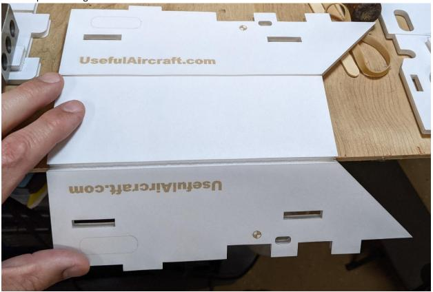
Next, take the avionics tray and apply hot glue to the interior bonding surfaces – not the tabs that will penetrate the fuselage skin.
