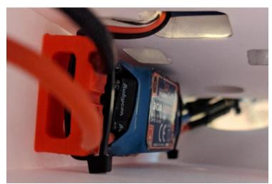
I float my ESCs using a 3D printed mount that secures to the interior side wall of the aircraft with hot glue. The mount allows for airflow all around the ESC for better cooling in hot environments and demanding conditions. This keeps my ESC's away from the receiver and FPV equipment and seems to work well for reducing interference. It also keeps hot glue off my ESCs. ESCs can melt hot glue. Ask me how I know.
