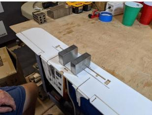
Unfold the wing, and use a popsicle stick to smear the hot glue along the top surface of the seam. Use weights to keep the wing flat while the Hot Glue cools.
