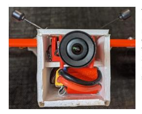
The battery compartment is designed to slip fit a 4s battery. It should hold it snug. The battery must be pushed back far enough to allow the Nose Slip Ring to engage the leading edge of the fuselage. I routinely fly this with various 4S batteries from 1300mah to 2200mah. 3S and Li-lon (either 18650 or 21700) packs will fit, but will require some additional means to prevent them from sliding around during flight.
