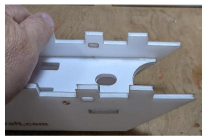
The forward set of tabs has a cut out for wiring to pass through.
