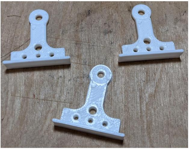
Push the control horn through from the underside of the elevator and ailerons. Apply hot glue and allow it to cool. Control horns are 3d printed and too much heat could deform them, so allow the horns to cool fully before flipping the airplane and applying more glue.
