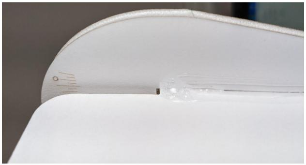
Once the hot glue has cooled and set, we need to secure the elevator at the outer face of the vertical stabilizers as shown in the photo below. This second bead of hot glue prevents vibration from simply delaminating the foamboard on the surface of the vertical stabilizers. This is done by a simple bead of hot glue at the exterior junction of the tabs and the vertical stabilizer. Perform this step on both the left and right sides.
