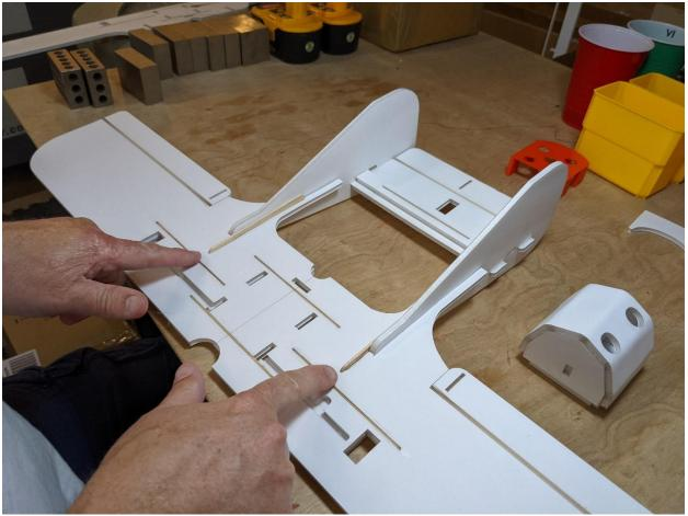
As further reinforcement, I run beads of hot glue down all mating surface joints. This is a good idea to do at all 90 degree joints on your airframe.
