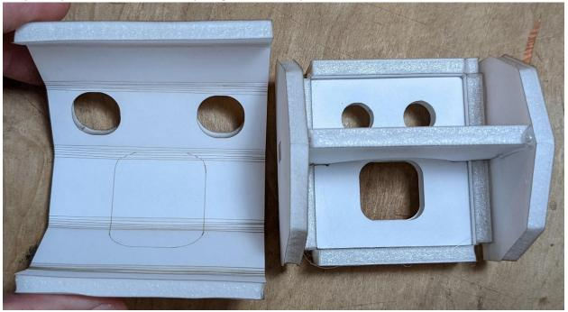
When ready, apply hot glue to on all edges of the Camera Platform, side skins, and the front half of the slip ring. The back half of the slip ring will form a press fit into the fuselage, and that's why there's a line around the perimeter of the slip ring - to mark this boundary. Try not to get hot glue on the back half of the slip ring.
