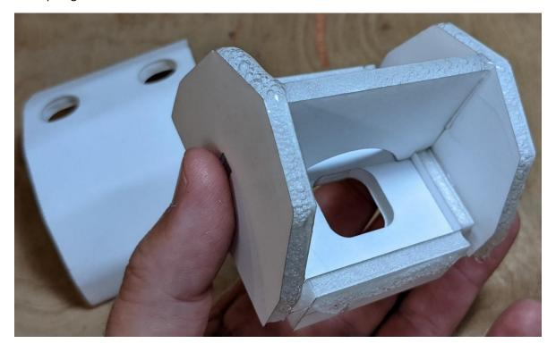
At that point, and referencing the Nose Frame, install the Nose Skin to match the Nose Frame.
