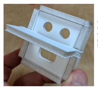
The Nose Frame is not glued in. It is simply used to hold the Slip Ring square and the camera tray flat during the rest of the installation. It also provides a guide to show how to install the Nose Skin (match the air inlets and camera ports).
