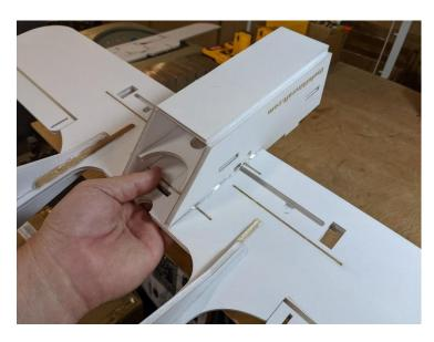
Run a bead of hot glue down the wing to fuselage juncture to further ensure a solid mating.
