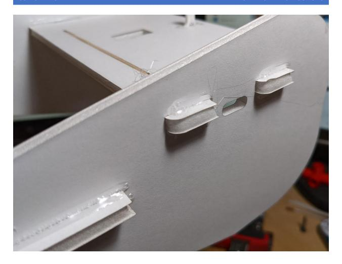
Ensure the elevator tabs are glued on the outside of both vertical stabilizers as shown in the photo above. All 4 tabs protruding through the vertical stabilizers should be glued from above and below.
