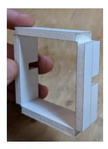
The Slip Ring is glued in this position, and in the photo to the left, I'm holding pressure on the glue joint. Hold this pressure manually, keeping all parts in alignment, and allow it the glue to cool. Don't rush this.
