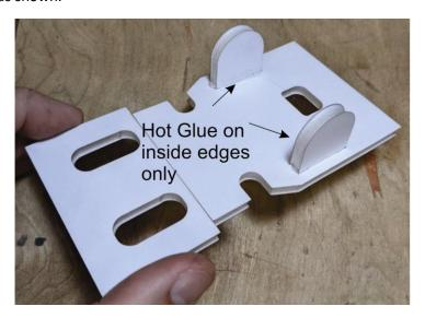
After completion of the build, if a more secure closing of the hatch is required, hot glue can be added to the exterior surfaces of these tabs as shown below. Check this prior to first flight.
