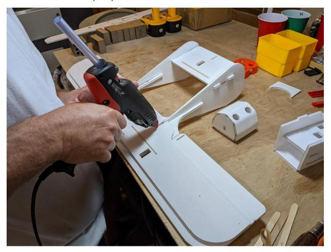
When fully mated, flip the wings and tail over, so we can now work on the underside. We need to install the popsicle sticks that will help to distribute pitching moments. I point out where those go in the photo below.
