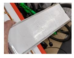
I apply clear packing tape to the underside of my fuselage, overlapping from back to front. It acts as a second skin and helps to prevent damage to the foamboard on landings on damp surfaces, grass, sand, dirt, and even asphalt.
