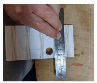
Use the straight edge to keep the foamboard rigid as you form the folds. The straight edge is placed behind the last fold line in any given group. The foamboard is held firmly against the straight edge and then bent a little more than 45 degrees. The foamboard will rebound after, closer to its original shape, and that's fine. We're just setting a prebend to make our final installation easier.
