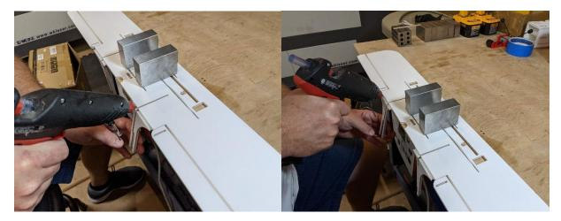
Once the Hot Glue is applied, Slide the wing forward onto the work surface and smear the Hot Glue along the fold seam. Repeat for both left and right sides. Allow the Lower Wing Skin to cool.
