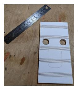
Find a ruler or a straight edge of some kind. We'll use this to make clean bends to the Nose Skin. The Nose Skin is pre-scored like the hinges that form the ailerons and elevators. In these cuts, the laser vaporizes the interior foam, allowing radius bends that leave the exterior skin intact.
