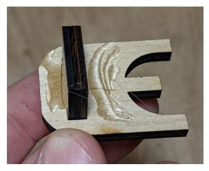
Apply hot glue as shown. Be sure to use enough glue that both the Alignment Pin and the motor mount are bonded.
