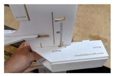
Ensure you are mounting the fuselage to the underside of the wing.
