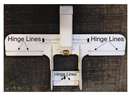
Insert the popsicle sticks into the lower wing skin. These will enhance the rigidity of the wing assembly and aid in alignment of the upper and lower wing skin.
